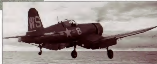
Below: An F4U-4 leaves the deck of a US Navy carrier. This major production version was intended to replace F4U-1s from 1945.
